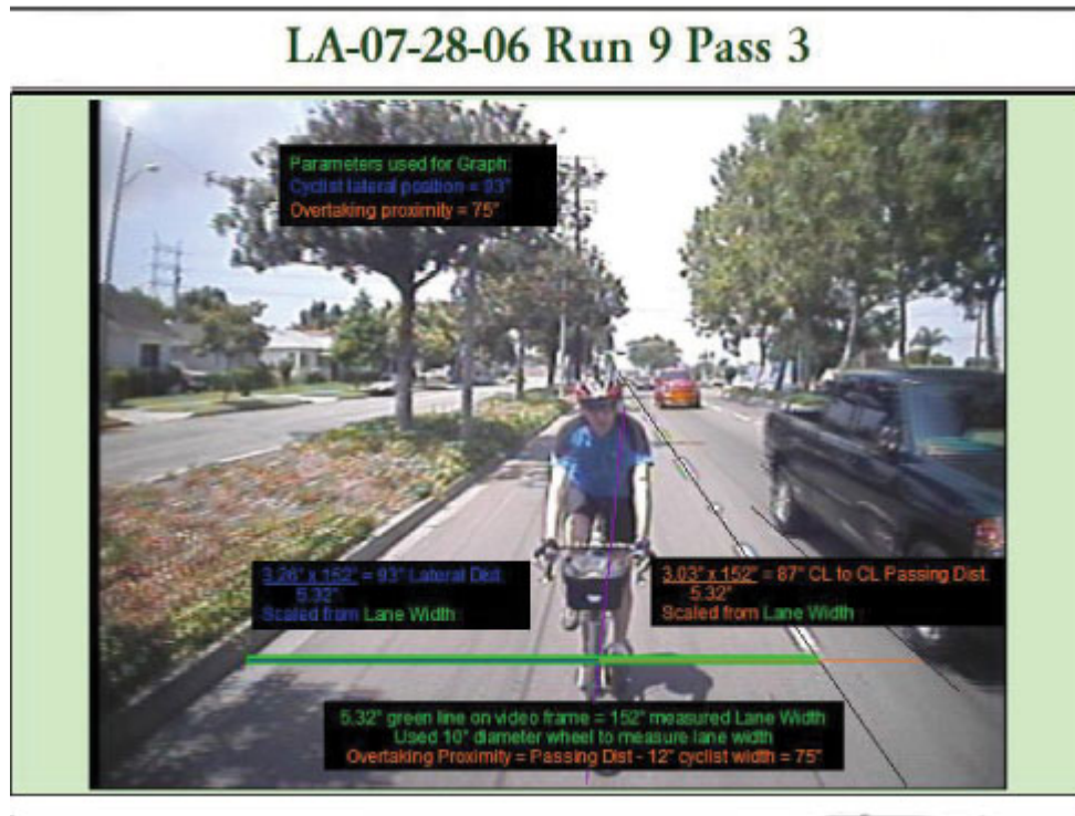
FIGURE 3 Example Still Image of Overtaking Maneuver with Measurements
